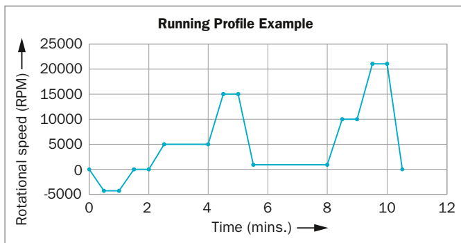
Figure 121: Example running profile showing varying rotational speeds throughout testing
