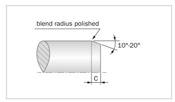
Figure 147 Lead-in chamfer on shaft
