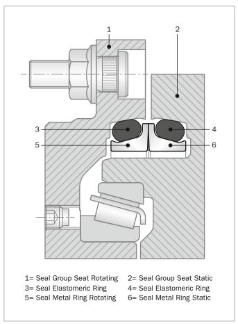
Figure 180: Mechanical Face Seals, Type DO
