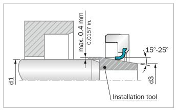
Figure 113: Fitting the sealing lip using an installation tool
