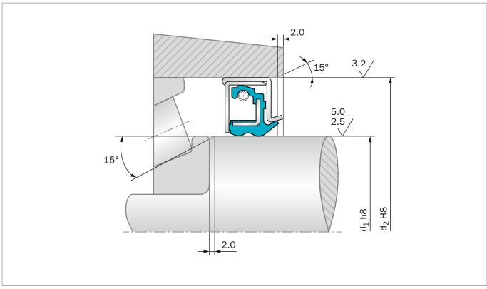
Figure 58: System 500 in wheel hub application (similar for System 2000 and System 3000)
