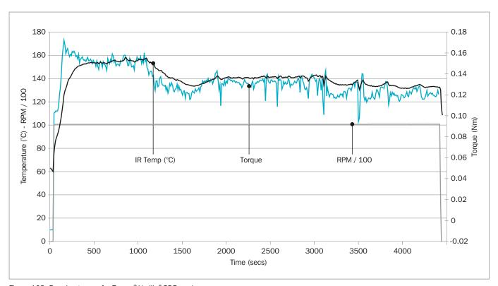
Figure 108: Running torque for Turcon® Varilip® PDR seals
