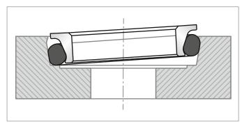
Figure 185: O-Ring slipped against the seat
