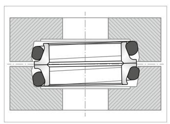
Figure 187: O-Rings slipped against seats and Mechanical Face Seal group is tilted
