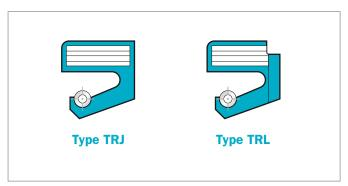
Figure 40: Fiber reinforced design for large diameters
