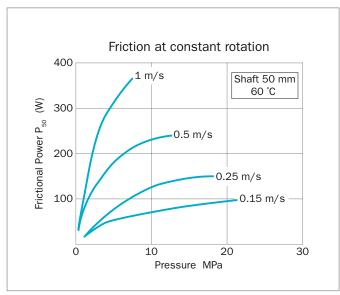
Figure 146 Frictional power for Turcon® Roto Variseal®
