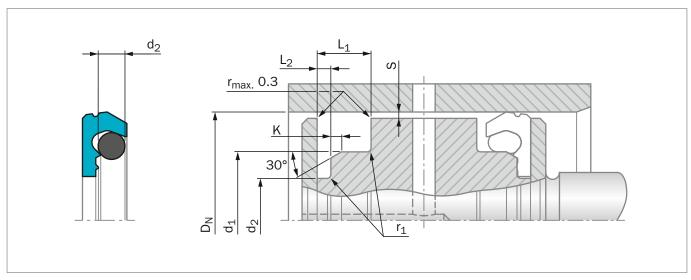
Figure 153: Installation Drawing
