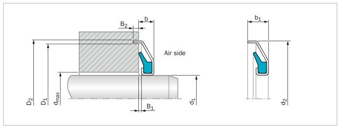
Figure 94: GAMMA seal with labyrinth
