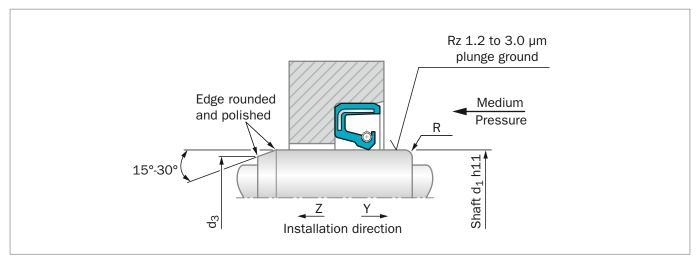
Figure 4: Installation of the Radial Oil Seal
