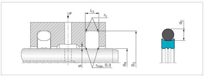
Figure 127: Installation Drawing
