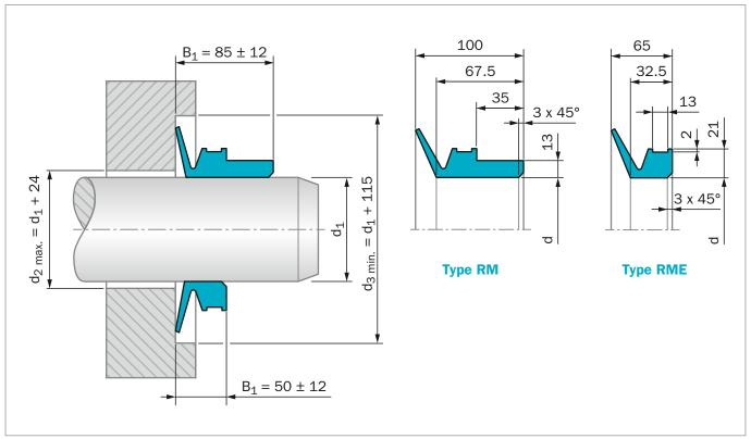
Figure 83: Installation Drawing
