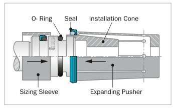
Figure 171: Calibration and installation of bore Turcon® Roto VL Seal® by an Installation Cone and Expanding Pusher
