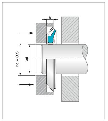
Figure 90: Assembly tool for TBP/RB
