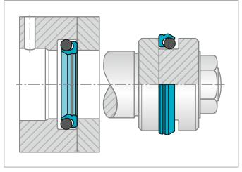
Figure 160: Installation of Roto VL Seal® in split grooves
