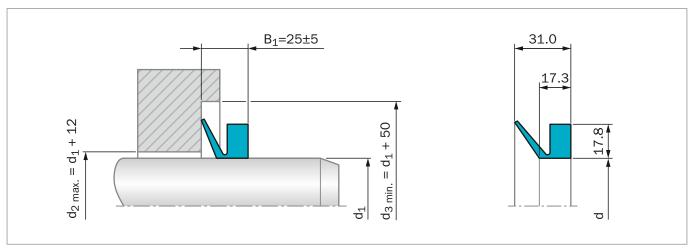
Figure 84: Installation Drawing
