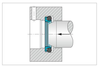
Figure 168: Direction of calibration of installed Roto VL Seal®
