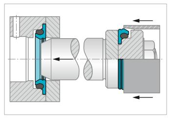
Figure 163: Installation of rod Turcon® Roto Variseal® and Roto VL Seal® F in split groove
