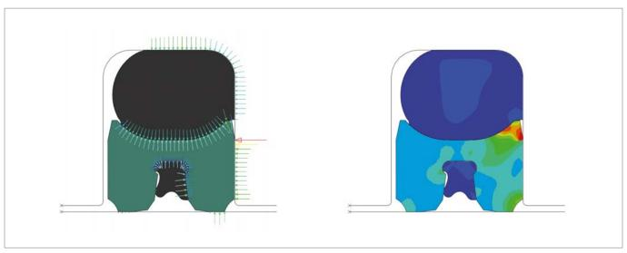
Figure 134 Turcon® Roto Glyd Ring® V - Finite Element Analysis (FEA).
