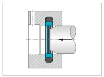
Figure 165: Calibration of installed Roto Glyd Ring®
