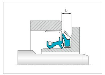
Figure 38: GAMMA seal fitted on the shaft boss
