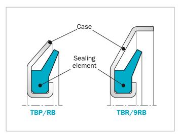
Figure 85: GAMMA seal types
