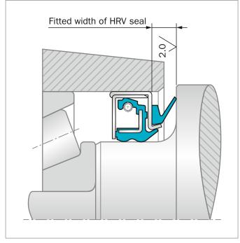
Figure 62: System 500 with HRV seal
