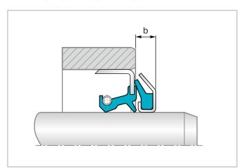
Figure 37: GAMMA seal fitted on the shaft end
