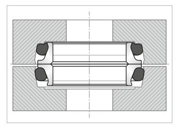
Figure 188: Upper half of the Mechancial Face Seal group has O-Ring slipped against the seat and on the seat bottom
