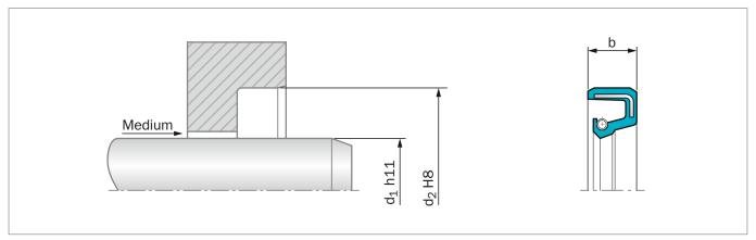
Figure 14: Installation Drawing
