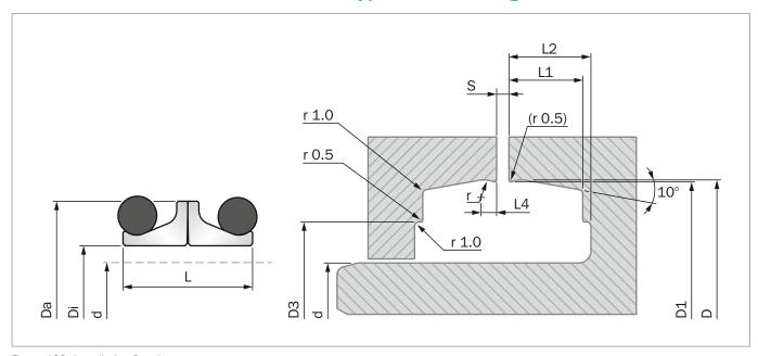
Figure 192: Installation Drawing
