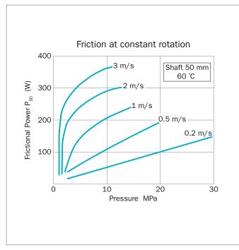
Figure 156: Frictional power for Turcon® Roto VL Seal®
