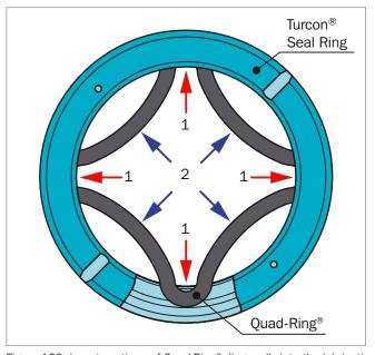
Figure 166: Insert sections of Quad-Ring $^{\circ}$  diagonally into the lubrication groove
