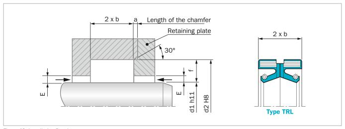
Figure 48: Installation Drawing
