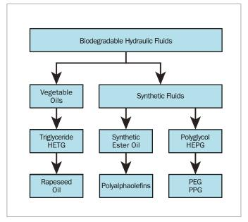
Figure 8: Biodegradable hydraulic fluids
