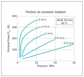
Figure 151: Frictional power for Turcon® VL Seal® F
