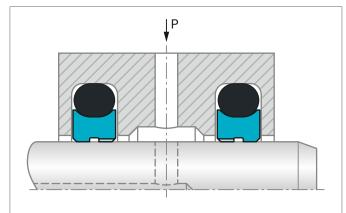
Figure 130: Right installation of Roto Glyd Ring $^{\circ}$  K
