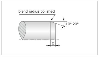
Figure 173: Lead-in chamfer on shaft
