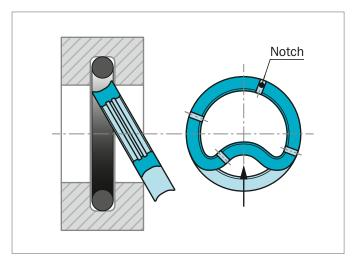
Figure 164: Installation of shaft Roto Glyd Ring® type in closed groove
