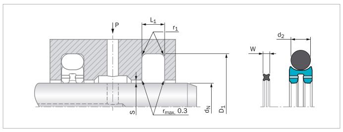
Figure 137 Installation Drawing
