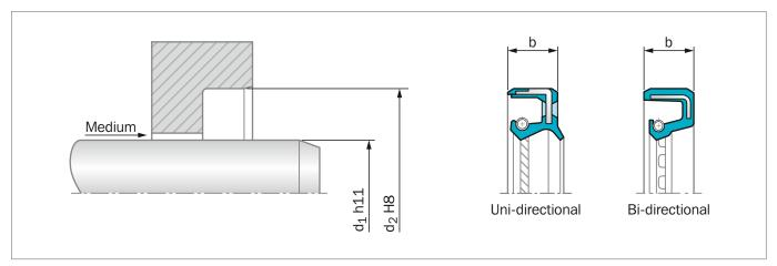
Figure 35: Installation Drawing
