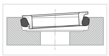
Figure 184: Metal ring slipped against the O-Ring
