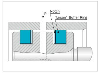
Figure 177: Right installation of Turcon® Buffer Ring
