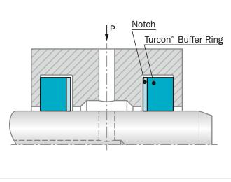
Figure 176: Right installation of Turcon® Buffer Ring
