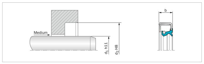
Figure 19: Installation Drawing
