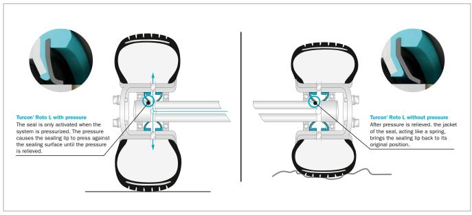
Figure 96: Functional Principle Turcon® Roto L
