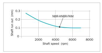
Figure 60: Permissible run-out of the shaft
