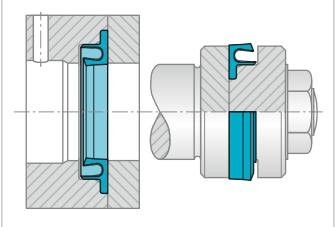
Figure 161: Installation of Variseal®
