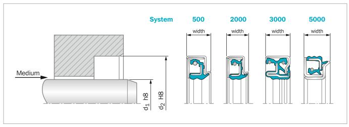
Figure 56: Installation Drawing
