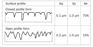
Figure 5: Examples of various surface profile parameters
