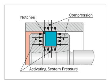
Figure 175: Pressure activation of Turcon® Buffer Ring
