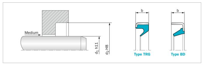
Figure 34: Installation Drawing
