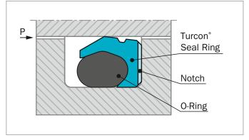
Figure 155: Turcon® Roto VL Seal® with radial notch
