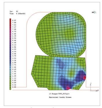
Figure 140  $\,$  Zurcon $^{\circ}$  Roto Glyd Ring $^{\circ}$  S - Finite Element Analysis (FEA)
