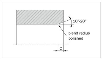
Figure 174: Lead-in chamfer on housing
