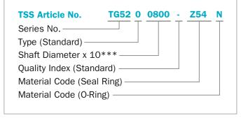
\*\*\* For diameters  $\geq$  1,000.0 mm multiply only by factor 1.
