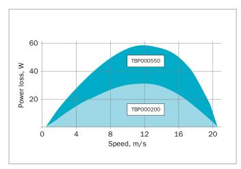
Figure 86: Power loss as a function of peripheral speed (Counterface 1.5 - 2  $\mu$ m Ra not lubricated seal)
