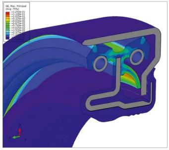
Figure 53: Friction optimization through FEA
