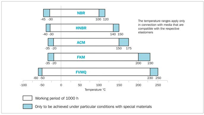
Figure 7: Temperature limits for some common types of rubber
