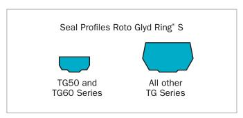
Figure 141 Cross-section profiles depending on Series No.
