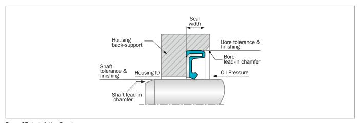
Figure 27: Installation Drawing
