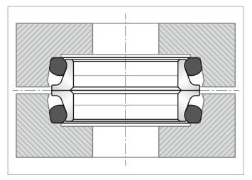
Figure 189: Both halves of the Mechanical Face Seal group have 0-Rings slipped against the seat and on the seat bottom
