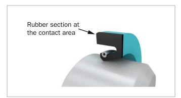
Figure 41: Contact area, split seal
