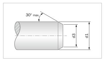
Figure 112: Shaft lead-in chamfer
