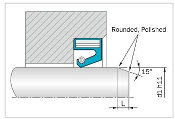
Figure 44: Installation of the oil seal
