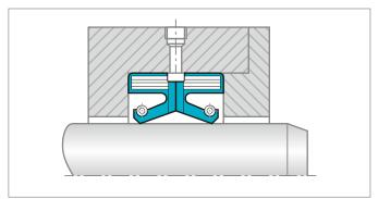
Figure 42: Type TRL mounted back to back
