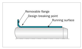
Figure 69: Design of the shaft repair kit
