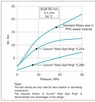
Figure 142 Friction of seals after endurance test
