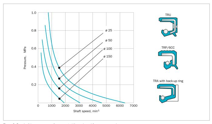
Figure 9: Permissible overpressure for supported lip seals and for pressure seals  $% \left( 1\right) =\left( 1\right) \left( 1\right)$
