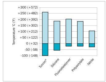
Figure 107: Maximum and minimum temperatures for different materials
