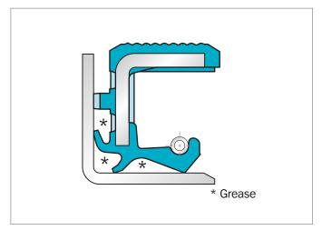
Figure 64: APJ for corrosive applications
