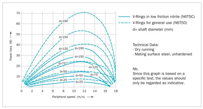
Figure 75: Power loss as a function of peripheral speed for various sizes
