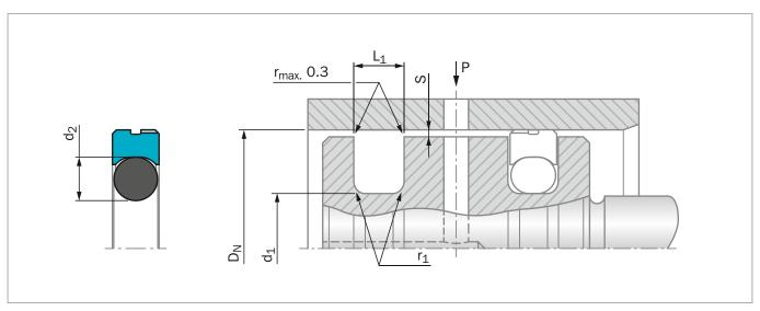
Figure 132: Installation Drawing
