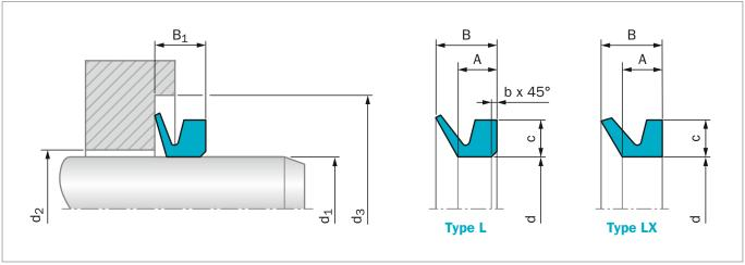
Figure 82: Installation Drawing
