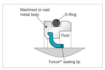
Figure 101: O-Ring Design. For low interference fits in the housing. Housing surface finish > 0.8  $\mu$ m Ra or particularly searching media control.
