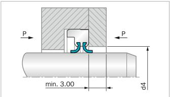
Figure 119: Installation type for fluid separation (Type D) at pressures up to 0.5 MPa (73 psi).
