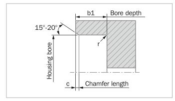
Figure 111: Housing design schematic
