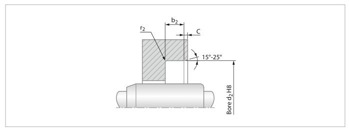
Figure 6: Installation depth and lead-in chamfer
