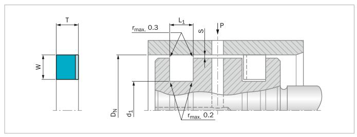
Figure 179: Installation Drawing
