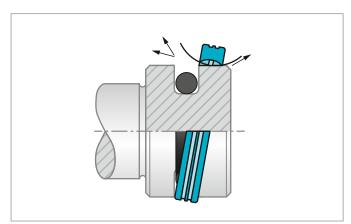
Figure 172: Schematic installation of the Turcon® seal ring
