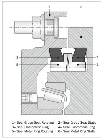
Figure 181: Mechanical Face Seals, Type DF
