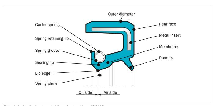
Figure 1: Designation for rotary shaft lip seals (extract from ISO 6194)  $\,$
