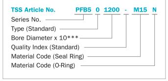
\*\*\* For diameters  $D_N \ge 1,000.0$  mm multiply by 1 Example: PFB8X for diameter  $D_N = 1,500.0$  mm Article No. PFB8**X1500**-M15
