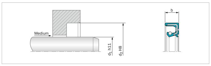
Figure 21: Installation Drawing
