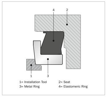
Figure 191: Installation Tool for DF Type
