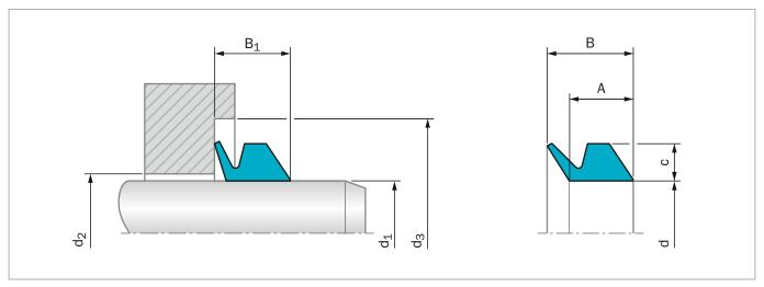
Figure 81: Installation Drawing
