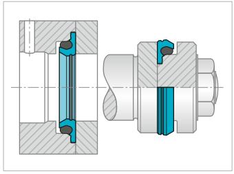
Figure 162: Installation of rod Turcon® Roto Variseal® and Roto VL Seal® F in split groove
