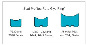
Figure 125: Crosssection profiles depending on Series No.
