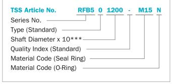
\*\*\* For diameters  $d_N \ge 1,000.0$  mm multiply by 1 Example: RFB8X for diameter  $d_N = 1,500.0$  mm Article No. RFB8**X1500**-M15
