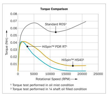
Figure 32: Torque comparison for HiSpin® products versus standard Radial Oil Seals.
