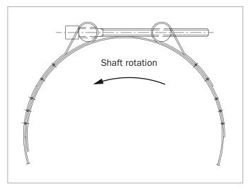
Figure 78: Clamping band RM
