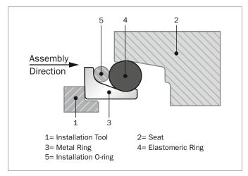
Figure 190: O-Ring as installation aid
