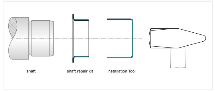
Figure 71: Installation sequence
