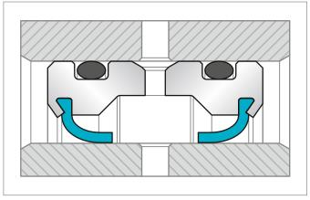
Figure 103: Fluid Transfer. Injection ports enable the transfer of fluid between the housing and the shaft.
