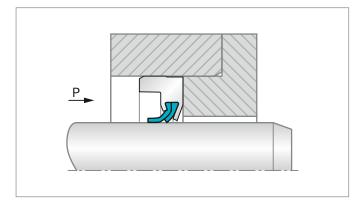
Figure 118: Installation for pressure from 0.5 MPa (73 psi) up to 1 MPa (145 psi). It is recommended to machine the housing to support the back of the seal.
