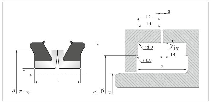
Figure 193: Installation Drawing
