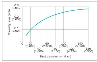
Figure 110: Coaxial tolerance capability
