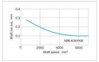
Figure 2: Shaft run out
