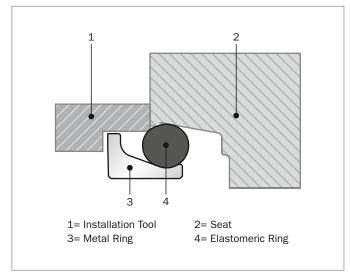
Figure 183: Installation Tool for DO Typel
