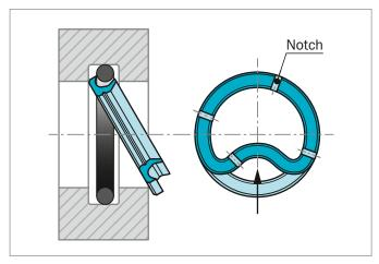
Figure 167: Installation of shaft Turcon® Roto VL Seal® in closed groove
