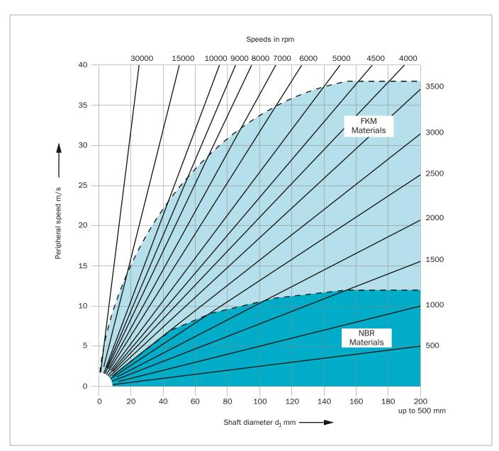
Figure 10: Permissible speeds in pressure-free state to DIN 3761
