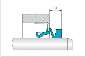
Figure 39: V-Ring fitted on the shaft end
