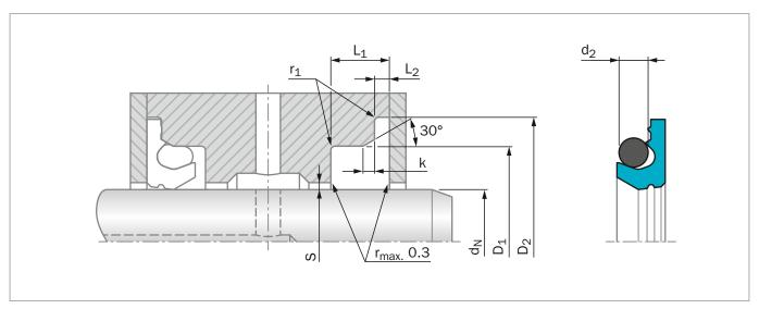
Figure 152: Installation Drawing
