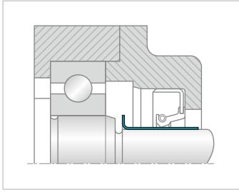
Figure 70: Running surface with shaft repair kit
