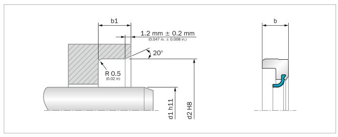
Figure 117: Installation drawing for pressures up to 0.5 MPa (73 psi)
