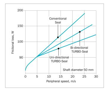
Figure 36: Friction loss
