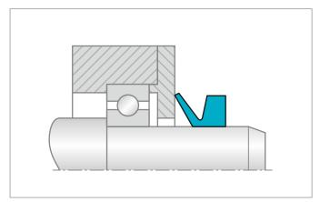
Figure 74: Method of operation of the V-Ring
