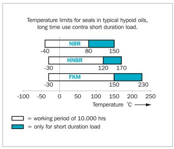
Figure 57: Temperature recommendations in typical hypoid oils
