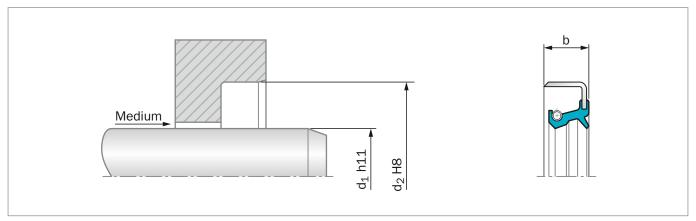
Figure 17: Installation Drawing
