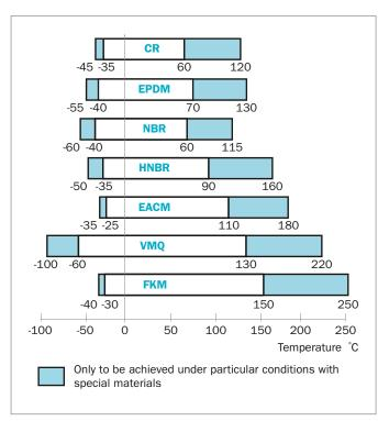
Figure 76: Temperature recommendations for V-Rings
