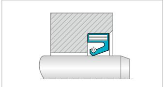
Figure 43: Type TRJ/F mounted without axial retaining plate
