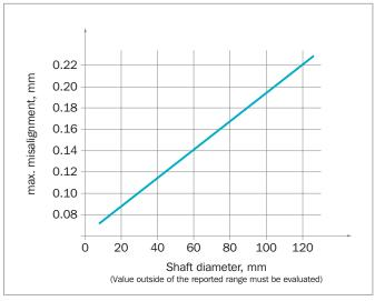
Figure 26: Shaft to bore misalignment
