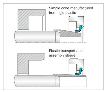
Figure 114: Assembly tooling types for installation on shafts
