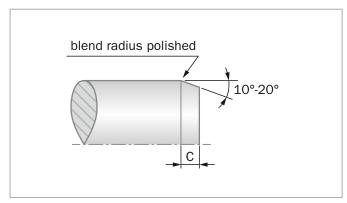
Figure 147 Lead-in chamfer on shaft
