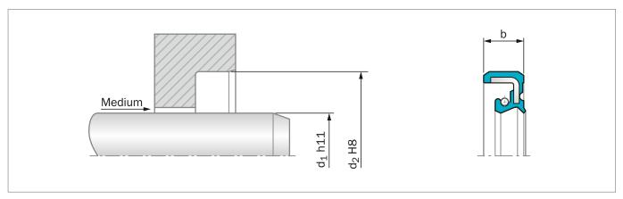
Figure 23: Installation Drawing
