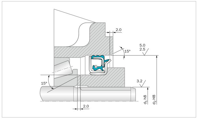
Figure 59: System 5000 in pinion application
