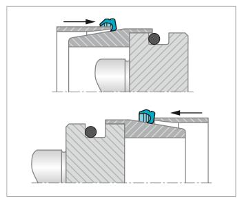
Figure 170: Installation of bore Turcon® Roto VL Seal® in closed groove using an expanding pusher over an installation cone
