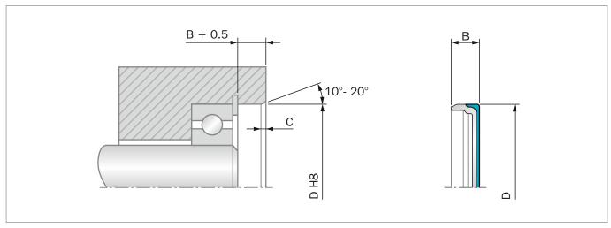
Figure 68: Installation Drawing
