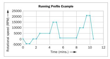
Figure 30: Example running profile showing varying rotational speeds throughout testing
