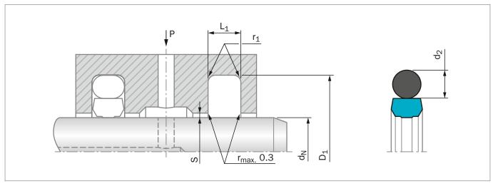
Figure 143 Installation Drawing
