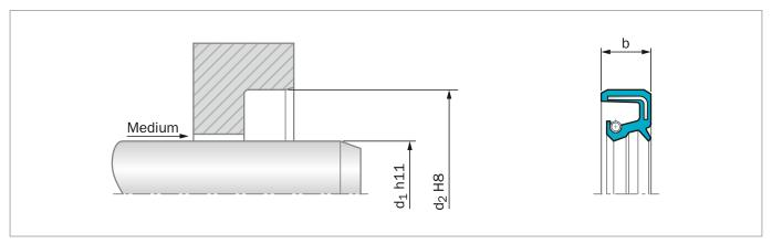
Figure 15: Installation Drawing
