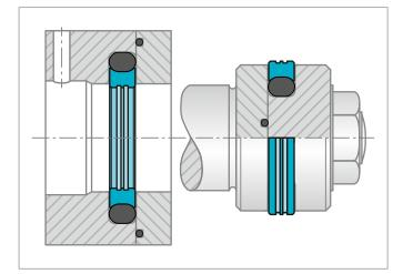
Figure 159: Installation of Roto Glyd Ring® in split groove
