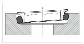
Figure 186: O-Ring slipped against the seat and waved against the metal ring
